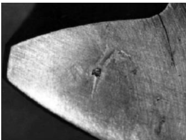
Bending Fatigue Crack
