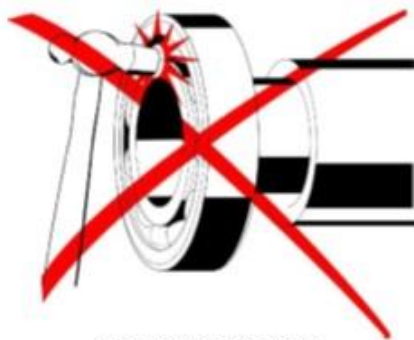
No Hammer Blows
