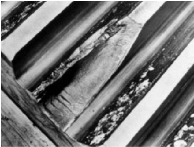
Profile Cracks Originating from Severe Pitting
